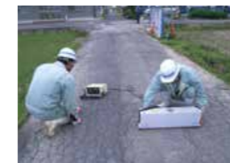
Position detection using the electromagnetic detection method
